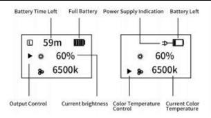
Power Supply indication: the icon will display when power is connected. Battery: Time left under current output, "m" stands for minute, "h" stands for hour. Current Output: Output under discharge condition.
